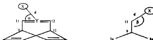
Figure 2. Definition of distance d and the angles \alpha and \beta ; X = Cl − , Br − and I −
